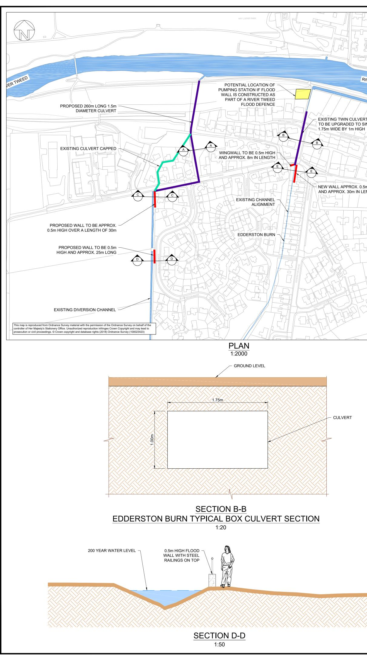
Peebles **Option 3C: South Parks** 200 Year Standard of RIVER TWEED Protection Culvert Upgrade WEIR With Direct Defences EXISTING TWIN CULVERT APPROX. 95m LONG TO BE UPGRADED TO SINGLE BOX CULVERT **GROUND LEVEL** NEW WALL APPROX. 0.5m HIGH AND APPROX. 30m IN LENGTH **SECTION A-A DIVERSION CULVERT TYPICAL SECTION** 1:20 0.5m HIGH FLOOD WALL WITH STEEL RAILINGS ON TOP 200 YEAR WATER LEVEL SECTION C-C 1:50 0.5m HIGH FLOOD WALL WITH -STEEL RAILINGS ON TOP 200 YEAR WATER LEVEL SECTION E-E 1:50
